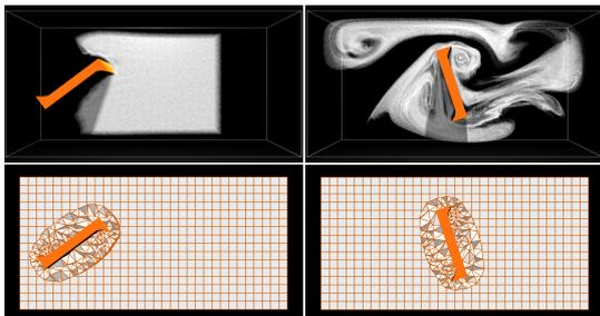
**Figure 1:** Top: A paddle mixes smoke in a tank. Bottom: A cross-section of the regular-tetrahedral bi-layer grid used.
